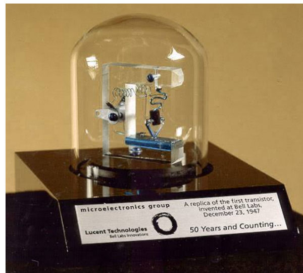
Figure 2.1: A 1997 commemorative replica of the first point-contact transistor, demonstrated at Bell Telephone Laboratories in December 1947. The photograph is a public-domain work of the Executive Office of the President of the United States, obtained through Wikimedia Commons .
